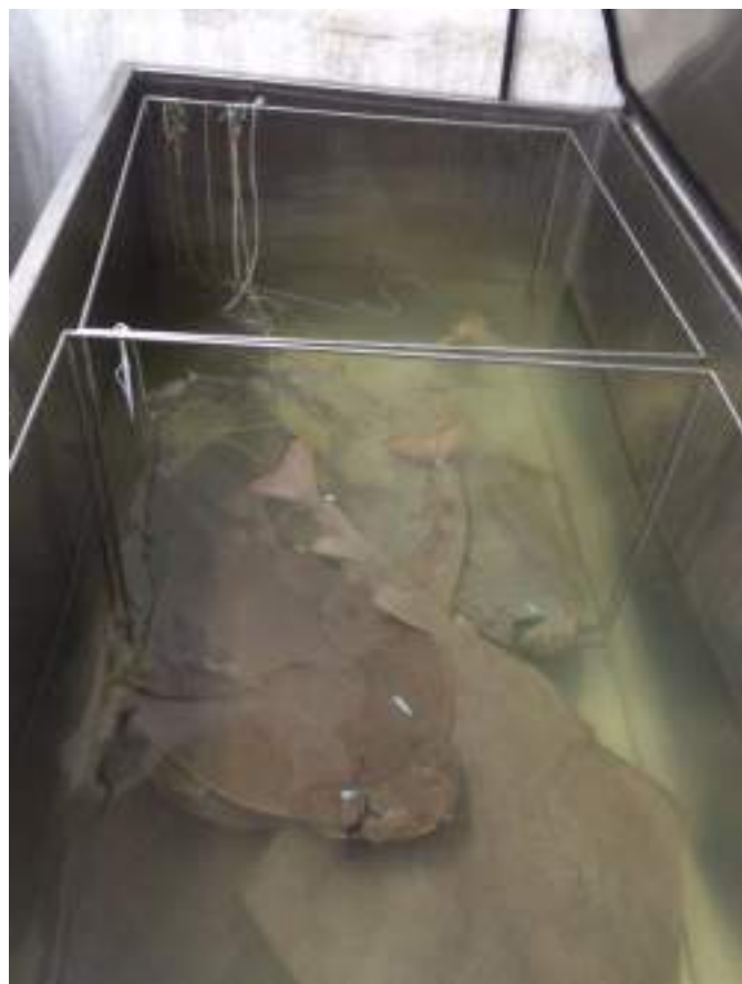
Figure 5. Stainless steel tanks used for storage of large specimens in the Ichthyological Collection of the Museu Nacional, Universidade Federal do Rio de Janeiro. Each 2,000 litre tank is equipped with internal railings for attachment of plastic labels connected with guide strings to the specimens.
